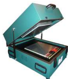
Fig. 1. Isothermal calorimeter for large prismatic cells
