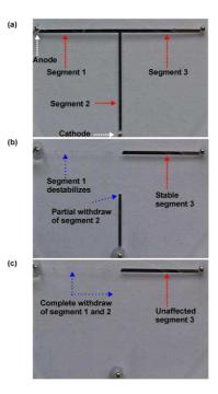
This reducing potential electrochemically removes the oxide and the metal instantaneously flows to the direction of the other electrode where it can minimize surface energy. We will also describe simple approaches to induce the liquid metal to flow into microchannels using modest voltages. Combinations of these two techniques are capable of producing electrochemically reversible and tunable sensors, actuators, RF antennas, Filters and micromixers.
