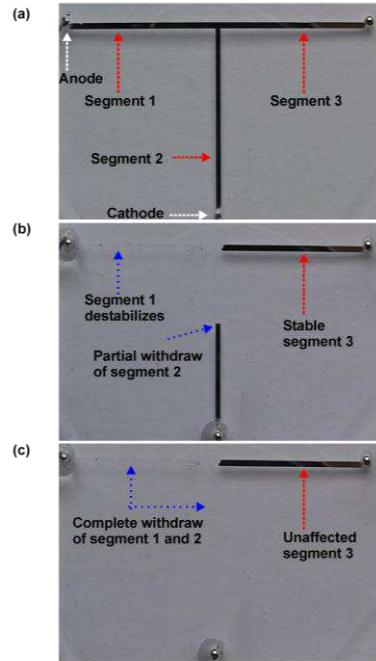
This reducing potential electrochemically removes the oxide and the metal instantaneously flows to the direction of the other electrode where it can minimize surface energy. We will also describe simple approaches to induce the liquid metal to flow into microchannels using modest voltages. Combinations of these two techniques are capable of producing electrochemically reversible and tunable sensors, actuators, RF antennas, Filters and micromixers.
