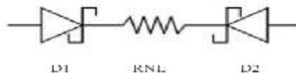
Fig. 1 A capacitor structure involving a high-k dielectric can be thought as two back-to-back Schottky diodes D1 and D2 with a non-linear resistor RNL in between.
