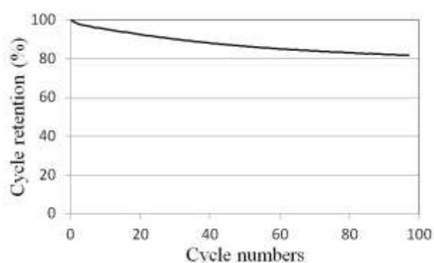
Figure 3. Cycle performance of 125mAh-class single cell at 60 °C.
