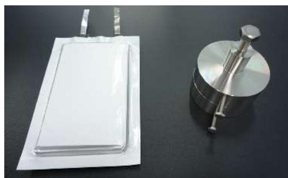
Figure 1. A large-size SSB (left) and a test cell (right).
