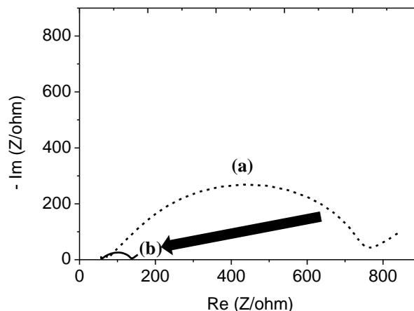
Figure 2. Nyquist plots of the test cells using (a) NCA and (b) LZO treated NCA for the cathode active materials at 25°C.
