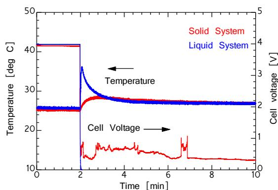
Fig.1 Cell voltages and surface temperatures both liquid and solid type LIBs during nail penetration test.
