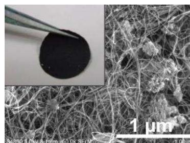
Figure 1. Photo and SEM images of a typical CNT-AC electrode.
