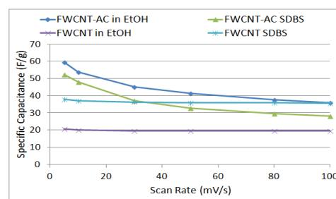
Figure 2. Galvanostatic rate capability of CNT-based self standing electrodes.
