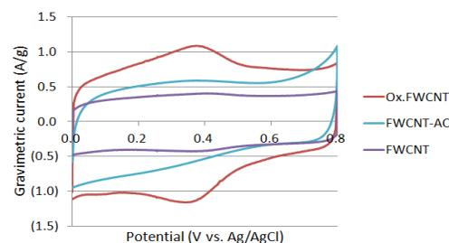
Figure 3. Cyclic voltammogram of FWCNT-based self standing electrodes. Scan rate: 10mV/s.
