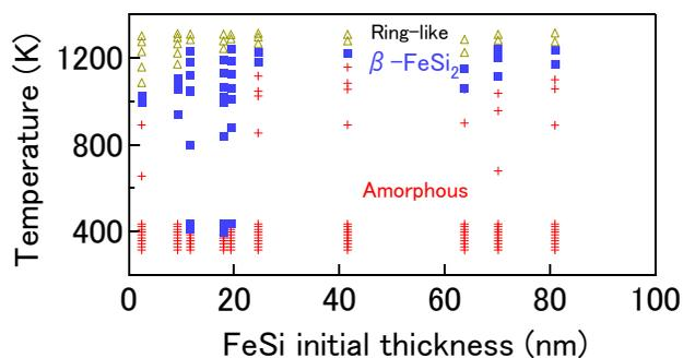
Fig1: Solid phase reaction on FeSi deposited Si(111) surface.
