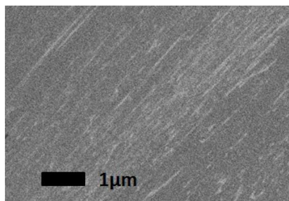
Fig.2: SEM image of  $\beta$ -FeSi<sub>2</sub> obtained with FeSi source. The initial deposition thickness of FeSi is 20nm. The SPG temperature was 397 K.
