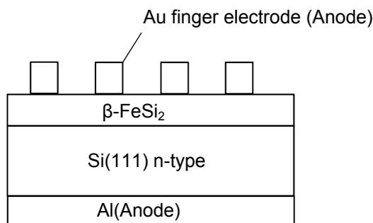
Fig.3: Test device structure for photo sensing.
