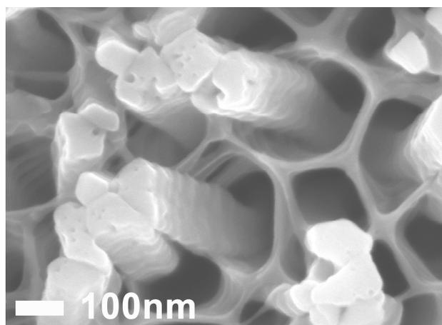
**Figure 1.** a) Synthesis of PEDOT inverse-nanotube-array and nanopore-array by selective electrodeposition with pulse current at 1.0 and 0.8 mA, respectively. The upper image represents titania nanotube electrode, the middle ones composites of titania and PEDOT, the lower images represent nanostructures of PEDOT obtained after dissolution of the template; b) SEM image of PEDOT inverse nanotube array.
