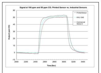
Figure 1. Comparison of response and achievement of steady state at commercial and printed amperometric sensors exposed to 50 ppm CO in air at room temperature.
