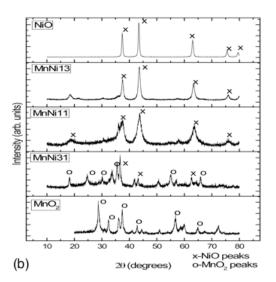
The presence of both layered and spinel structures in the cathode material were confirmed by the XRD pattern. Further results from ICP and SEM, TEM studies will be presented in detail during the presentation. The reverse micelle process facilitated the synthesis of uniform nano structured cathode materials.
