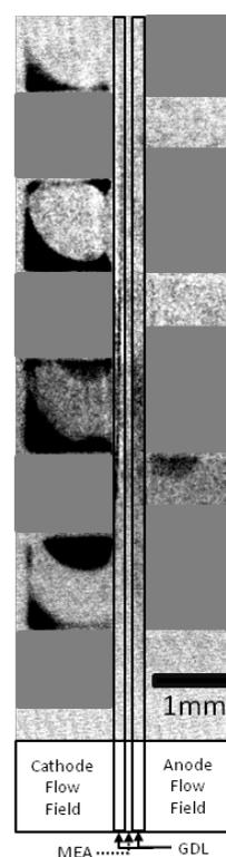
Figure 1: In-plane image of the PEM fuel cell. Solid grey regions are the ribs, and dark regions correspond to the presence of liquid water.
