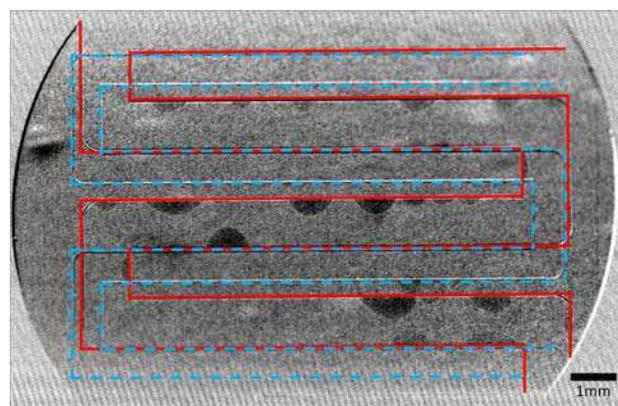
Figure 2: Through-plane image of the PEM fuel cell. The cathode channel is highlighted with solid red lines, and the anode channel is highlighted with dashed blue lines. The dark regions correspond to the presence of liquid water.
