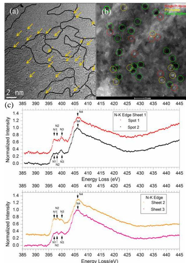
**Figure 1** ALD Pt on N-doped graphene. (a) HRTEM image of 150 ALD Pt cycles with black lines on graphene sheet edges and yellow arrows on Pt atoms and clusters. (b) HAADF image of 150 ALD Pt cycles with single Pt atoms, clusters of Pt atoms, and pits in the graphene labeled, and (c) N-K edge EEL spectra acquired from three graphene sheets.
