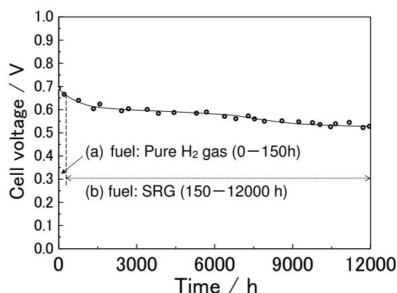
Fig. 1 Transition of cell voltage of a test cell during a continuous operation for 12000 h. Current density: 200 mA cm<sup>-2</sup>, Temperature: 80 °C, Humidity: 100% RH for anode and 66% RH for cathode.
