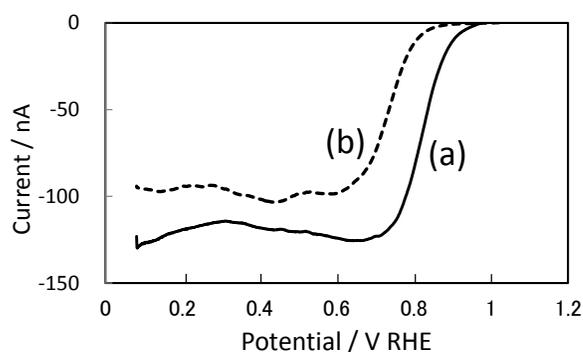
Fig. 3 i-E curves of ORR in O<sub>2</sub> saturated 0.5 mol dm<sup>-3</sup> H<sub>2</sub>SO<sub>4</sub> solution. (a): a catalyst of beginning operation, (b): a catalyst of 9000 hours operation. Scan rate of 1 mV s<sup>-1</sup>.
