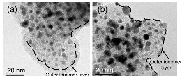
Fig. 2 TEM images of catalyst particles of cathode: (a) Initial stage, (b) After operation for 9000 h. The broken lines indicate outer ionomer layers of Pt-Co/C particles.
