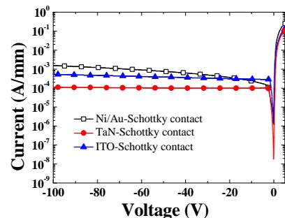
Fig. 3. Rectifying characteristics of AlGaIn/GaN SBDs for various Schottky contact
