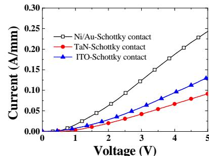
Fig. 2. Forward characteristics of AlGaIn/GaN SBDs for various Schottky contact
