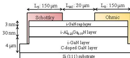
Fig. 1. Cross-sectional view of fabricated AlGaIn/GaN SBDs
