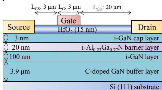
Fig. 1. Cross-sectional view of the fabricated AlGa<sub>0.23</sub>Ga<sub>0.77</sub>N MOS-HEMT with RF-sputtered HfO<sub>2</sub>
