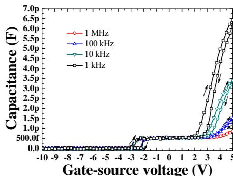
Fig. 3. Measured characteristics at frequency of 1, 10, 100 kHz, and 1 MHz with maximum gate bias of 5 V
