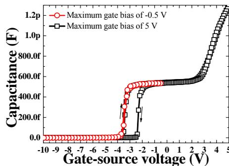
Fig. 2. Measured capacitance-voltage characteristics at 1 MHz
