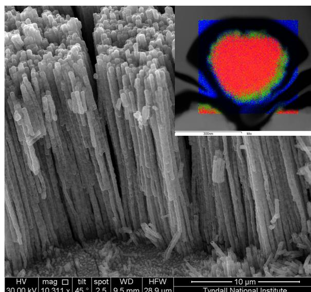
Fig. 1. SEM image of the core@shell Ni@NiO nanowire arrays. Inset: STEM-EDS elemental mapping shows the presence of a thin oxide layer around the Ni circumference: dark field (DF) image of core@shell Ni@NiO nanowire in which nickel at the inner core (red color) and oxygen at the outer shell (green color).
