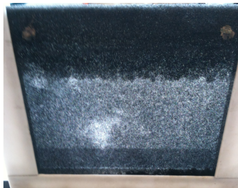
Fig. 1. The vitreous carbon foam anode, supported in a PTFE frame, showing the loss of carbon material which has been converted to GO.
