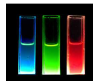
Fig. 1. Blue, green, and red light emission after illumination of 254-nm UV light for CdSe/ZnS QDs
