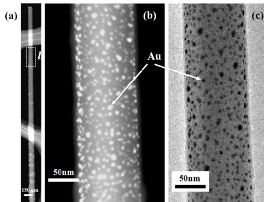
Fig.1 (a) HAADF-STEM image of Si-NW with the diameter of  $\sim 100$  nm annealed at 700°C using the standard furnace. (b) Magnified HAADF-STEM and (c) HR-TEM images of the Si-NW in the middle part *l* of (a). The bright spot in HAADF-STEM and black one show the Au NPs.
