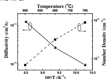
Fig. 2 Diffusivity and number density of Au NP with each annealing temperature exhibit an Arrhenius dependence on temperature.
