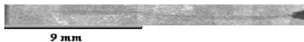
Fig. 1. BSE micrograph of UD-165 after a fatigue test in NaCl/NaHCO 3 /Na 2 CO 3 /p H 2 S = 0.83 kPa at 85°C, pH=7.
