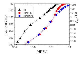
Hydrogen pressure–composition (PC) obtained electrochemically in 0.1M HClO<sub>4</sub> for pure palladium and Pd-N electrodes.
