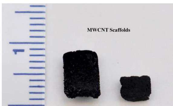
Figure 2: Optical images of purified MWCNT scaffolds prepared as cylinders (5 mm diameter, 8 mm length), and disks (5 mm diameter, 4 mm thickness).
