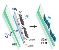
Designing semiconductor-Graphene Oxide-Metal Nanoparticles for SERS substrate. Photogenerated electrons in TiO<sub>2</sub> are transferred across GO film to deposit Ag nanoparticles in a controlled fashion.
