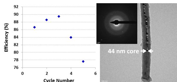
Figure 2. Coulombic efficiency as a function of cycle number calculated from the curves in Fig.1. An image of and diffraction pattern from the immersed portion of this Si nanowire cycled at 1.4C.
