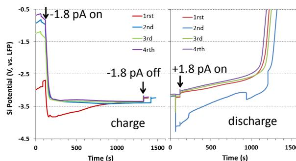
Figure 1. Charge and discharge curves for a 9.5 μm length of a 140 nm diameter Si nanowire cycled at a 1.4C rate
