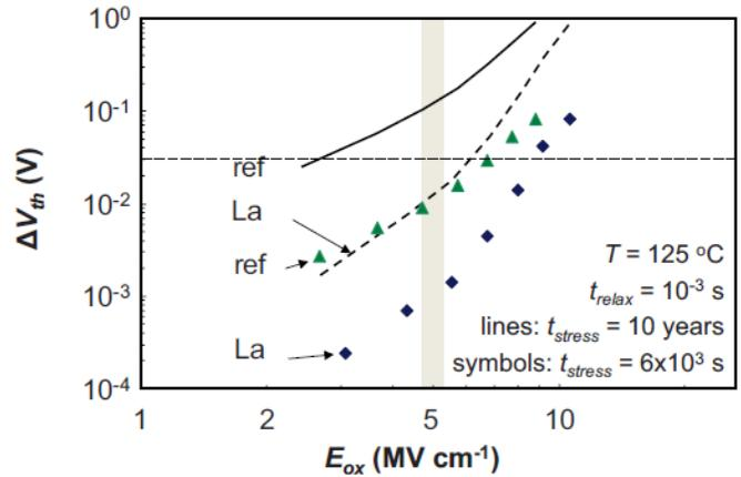
Fig. 1 Adding Lanthanum to Hf based dielectrics significantly reduces PBTI, improving the projection by > 5x. from [1]
