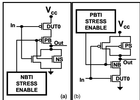
Fig. 3 Specialized RO structures. (a) NOR style circuit that stresses only the PFET DUT. (b) NAND style circuit that stresses only the NFET DUT. from [5]
