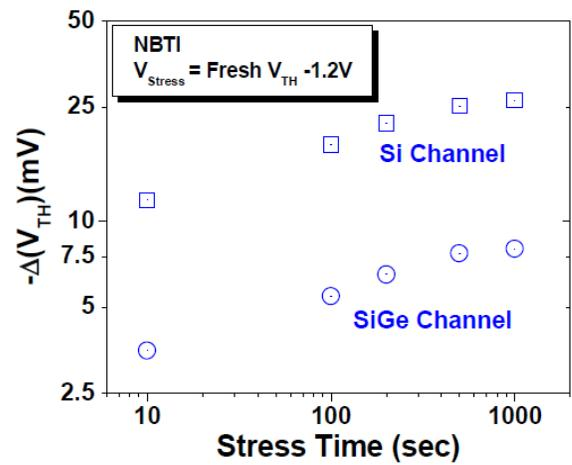
Fig. 2 NBTI can be improved significantly with a SiGe channel as compared to a traditional Silicon channel. from [2]
