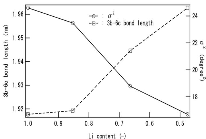
Fig. 2 Change of the 3b-6c bond length and the bond angle variance,  $\sigma^2$  with charge depth by neutron diffraction.
