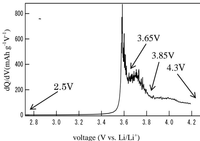
Fig.1 Differential capacity vs. voltage of  $\text{LiNi}_{0.8}\text{Co}_{0.2}\text{O}_2$  cell cycled in 2.5-4.3V charge.
