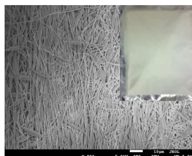
Fig. 1. SEM and digital (inset) images of a PFO-PEO fiber composite membrane prepared by the electrospinning technique.
