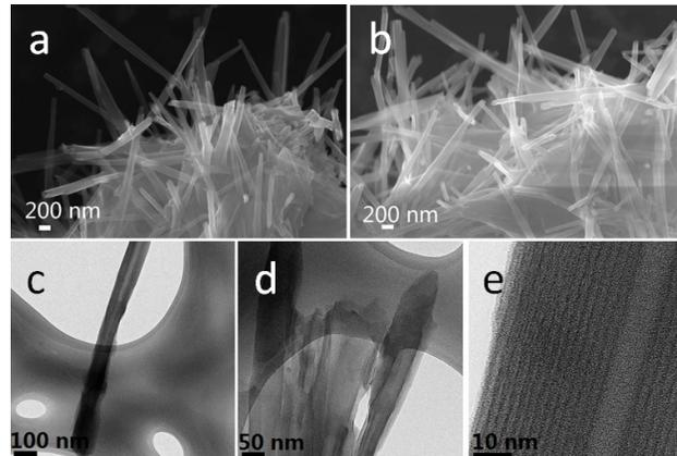
Figure 2. SEM and TEM image of the as-prepared vanadium oxide nanotube
