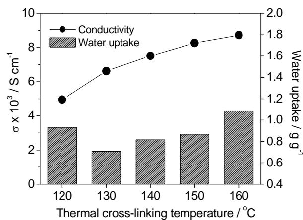
Fig. 2 Cl<sup>-</sup> conductivity and WU of PVA/PDDA/MWCNTs (1 wt.%) as a function of thermal cross-linking temperature. Polymer composition PVA/PDDA = 1:0.5 by mass.
