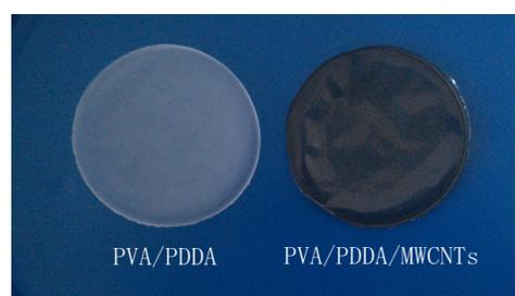
Fig. 1 Membrane pictures of PVA/PDDA membrane and PVA/PDDA/MWCNTs (1 wt.%) membrane. Polymer composition: PVA/PDDA = 1:0.5 by mass.
