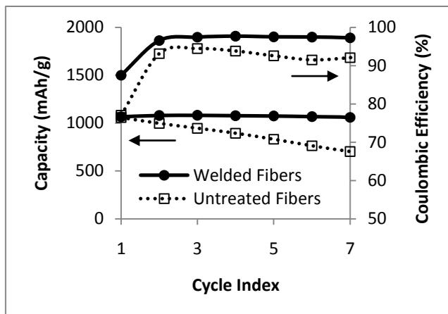
**Figure 1.** Electrochemical performance of Si based nanofiber anodes with and without a post-spinning welding treatment.
