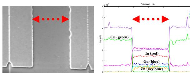
**Figure 3.** Auger line-scan of an IGZO TFT channel etched in an aqueous solution of (i) 5 wt. % citric acid and 2.5 wt. % hydrogen peroxide at 40 °C, followed by (ii) a 50 °C heated mixture containing 80 vol.% hydrogen peroxide solution and 20 vol.% containing TMA. The intensity of the Cu and Mo signal is zero (noise level) across the entire channel length. Mo signal at the S/D contact is also zero due to the thickness of the Cu metal.
