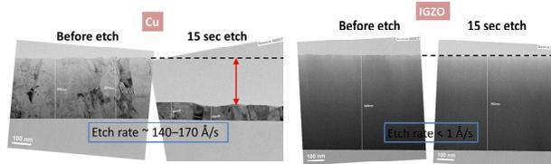
**Figure 2.** Cross-section TEM images of blanket Cu and IGZO films etched in an aqueous solution of 5 wt. % citric acid and 2.5 wt. % hydrogen peroxide at 50 °C.
