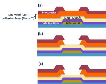
**Figure 1.** Schematic depicting our wet-etch process approach of (a) an IGZO TFT. First, the metal conductor (Cu) is selectively removed (b), followed by the metal adhesion layer (Mo or Ti), (c).
