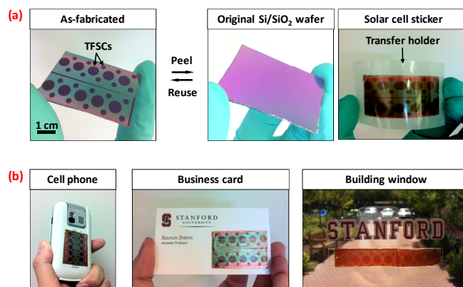
Figure 2: Thin film solar cells (TFSCs) at different stages of the peel-and-stick process. (a) As-fabricated TFSCs on the original Ni coated Si/SiO 2 wafer (left). The donor Si/SiO 2 wafer is clean and reusable after the peeling-off step (middle). The TFSCs are held by a temporary transfer holder (right). (b) TFSCs on cell phone (left), business card (middle), and building window (right).
