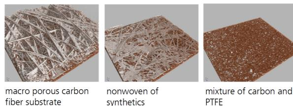
Fig. 1: 3D micrograph visualization of in-house GDL by computer tomography
