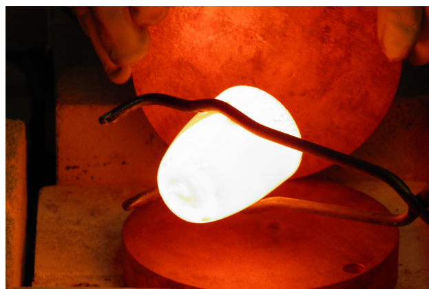
FIG. 1. Splat quenching an iron phosphate glass melt (glass melt in glowing hot crucible about to be poured onto bottom copper chill plate)
