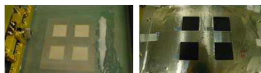
Figure 2. Thixotropic gel polymer electrolytes which is directly screen-printed on the electrode surface
