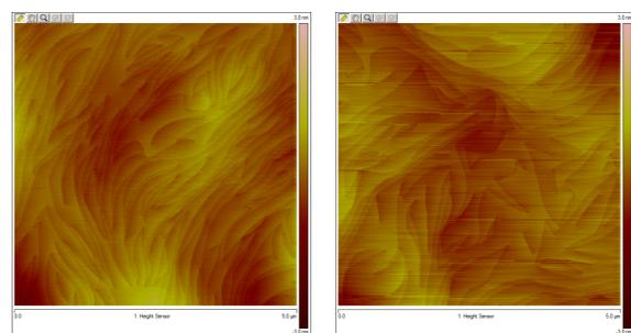
Figure 2. Identical surface morphology (RMS  $< 0.5 \text{nm}$  for  $5 \mu\text{m} \times 5 \mu\text{m}$  scan) with pseudomorphic growth mode for run-to-run and wafer-to-wafer.
