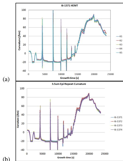
Figure 1. (a) wafer-to-wafer reproducibility and (b) run-to-run repeatability/stability for 6" HEMT runs.
