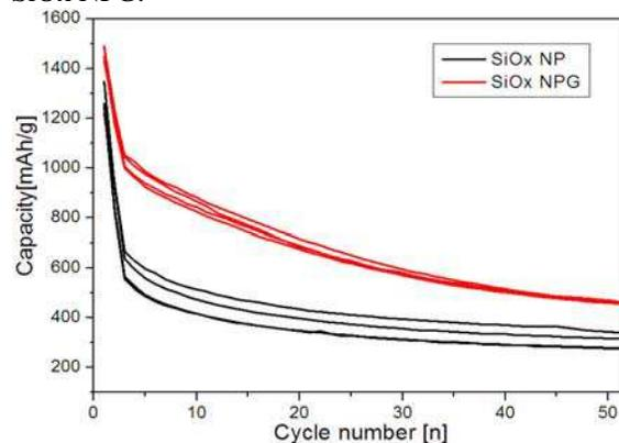
Fig. 4. Comparison of cycle performances of SiO<sub>x</sub> NP and SiO<sub>x</sub> NPG.
