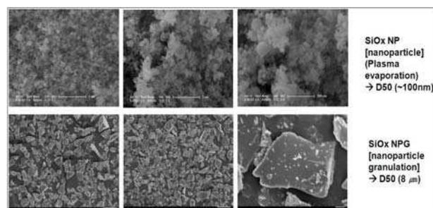
Fig. 2. SEM images of the SiO<sub>x</sub> NP and SiO<sub>x</sub> NPG; before and after granulation.
