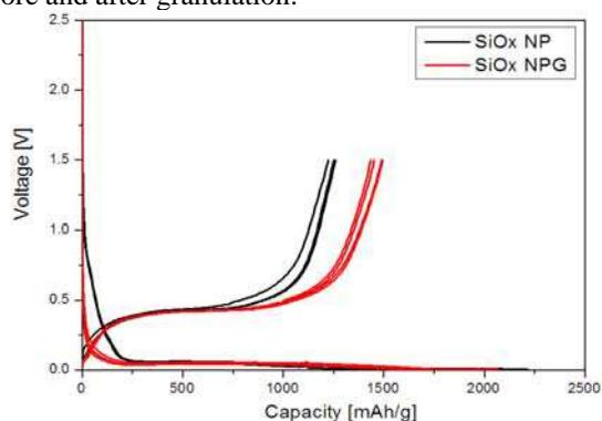
Fig. 3. Initial charge-discharge curves of SiO<sub>x</sub> NP and SiO<sub>x</sub> NPG.
