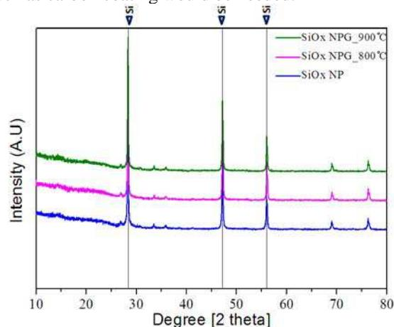
Fig. 1. XRD patterns of the as-fabricated SiO<sub>x</sub> nanoparticles [SiO<sub>x</sub> NP] and water granulated particles [SiO<sub>x</sub> NPG]
