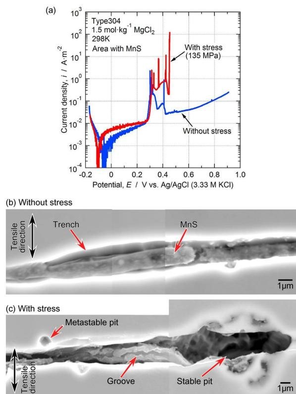
Fig.1 (a) Effect of stress on microscopic polarization curves for the small areas with MnS inclusion in 1.5 mol kg<sup>-1</sup> MgCl<sub>2</sub> at 298 K. (b, c) SEM images of the inclusions after the polarization measurements: (b) with stress and (c) without stress.
