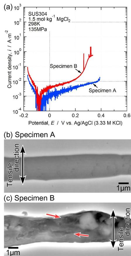
Fig.2 Effect of electrode potential on MnS morphology with applied stress. (a) Microscopic polarization curves for the small areas with the inclusion in 1.5 mol kg<sup>-1</sup> MgCl<sub>2</sub> at 298 K. (b, c) SEM images of the inclusions after the polarization measurements. The arrows indicate the grooves.
