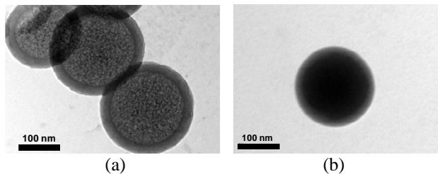
**Figure 1.** Transmission Electron Microscopy (TEM), SEM, images of the precursor carbon spheres (a) and of the hollow carbon sphere-sulphur composite (b).
