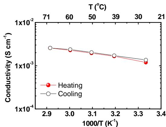
**Figure 3.** Arrhenius plots of conductivity of the TEGDME<sub>4</sub>NaCF<sub>3</sub>SO<sub>3</sub> electrolyte.
