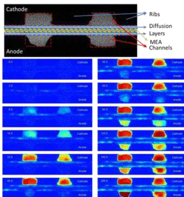
Figure 3. Gas evolution sequence in two channels in RFC in electrolysis mode
