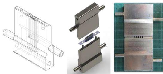
Figure 1. The cell design used in soft X-Ray visualization
