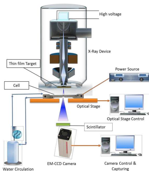
Figure 2. Soft X-Ray experimental setup for through plane visualization
