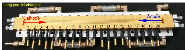
**Figure 1.** Flow-field plate of a segmented PEM fuel cell, divided into 20 segments along the channel length (active area 1 by 30 cm; 5 parallel channels).
