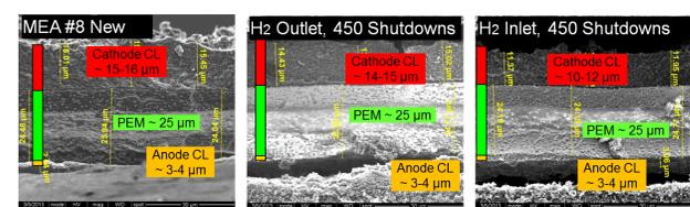
**Figure 3.** SEM images of non-uniform thinning of the cathode catalyst layer caused by shutdown aging protocol (MEA #8).
