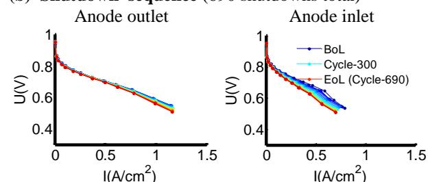
**Figure 2.** Time evolution of local polarizations curves for individual segments (anode outlet vs. inlet) during (a) startup and (b) shutdown aging protocols (MEA #6).
