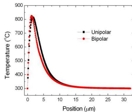
Fig. 1. Simulated temperature profiles of unipolar and bipolar switching in Cu/TaO<sub>x</sub>/Pt resistive memory devices.
