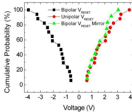
Fig. 2. Cumulative probability of RESET voltages of bipolar and unipolar switching for Cu filament.
