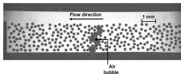
Figure 3: Greyscale image of the breakthrough moment for the microfluidic chip representing the felt GDL.
