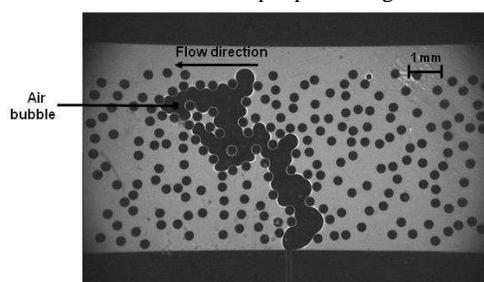
Figure 4: Greyscale image of the breakthrough moment for the microfluidic chip representing the foam GDL.
