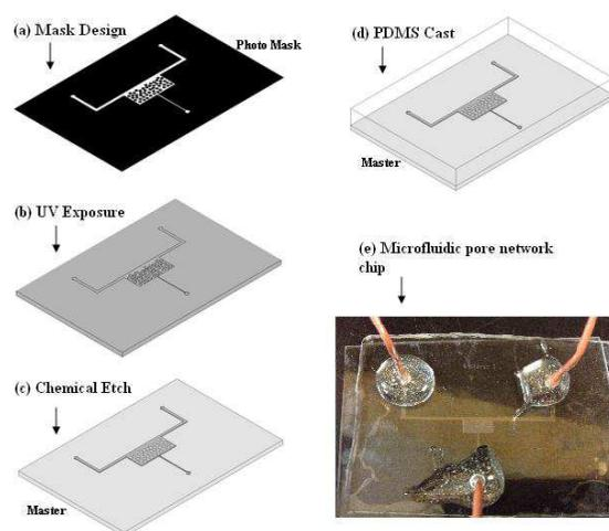
Figure 1. Fabrication procedure for a microfluidic chip (a) A photomask is produced. (b) A flat substrate coated with a thin photoresist layer is exposed to UV light. (c) Unexposed photoresist is chemically etched away, leaving a planar 3D pore network structure (master). (d) A PDMS elastomeric replica of master is cast (e) Cured PDMS is bonded to a glass slide to make the microfluidic chip.
