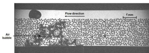
Figure 2: Greyscale image of the breakthrough moment for the microfluidic chip representing the sintered powder GDL.
