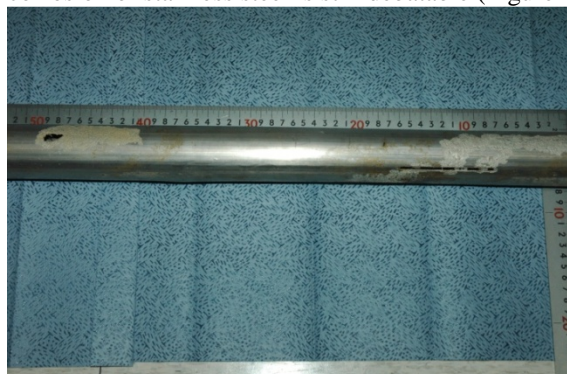
Figure 1. STS 304 pipe Leak by Corrosion after 2 Years of Service.
