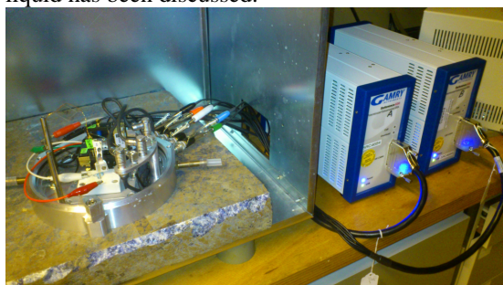
Figure 1. A SECM working station integrated with high speed digital bi-potentiostat (Gamry, US) for the detection of reaction intermediates.
