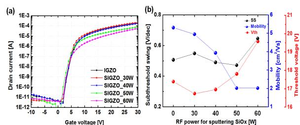
Fig. 1. (a) The representative transfer characteristics of various sputtering powers of TFTs and (b) extracted subthreshold swing (S.S.), mobility and threshold voltage with various Si concentrations.
