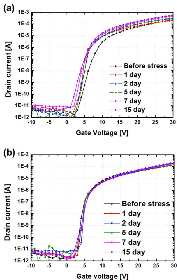
Fig. 2. Change of transfer curve between (a) conventional a-IGZO TFT and (b) a-IGZO/a-SIGZO double layered TFT under 50% relative humidity/50°C temperature condition for 15days.
