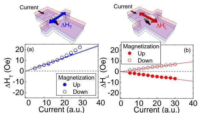
Fig. 2. Current induced effective field measured as a function of the input current[5]. Effective field transverse ( $\Delta H_T$ ) and along ( $\Delta H_L$ ) the current flow are measured for magnetization oriented normal to the film normal. Open and solid symbols indicate the magnetization direction.
