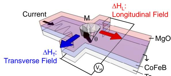
Fig. 1. Schematic illustration of the experimental setup used to measure current induced effective fields.
