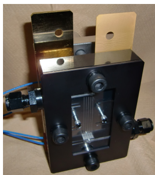
Fig. 1 See-Through PEFC with straight flow channels at the cathode.
