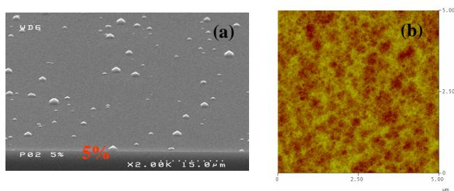
Fig.2. (a) SEM image of a textured silicon surface after immersion in a 5% diluted TMAH solution. (b) AFM 5µm<sup>2</sup> scan of a non textured silicon surface after 25% TMAH exposure.
