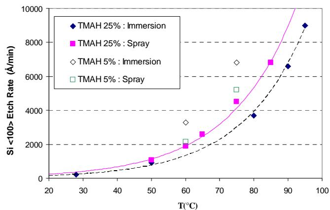
Fig.1. Influence of both chemistry dispense mode (immersion or spin-on) and TMAH dilution on the kinetic of silicon wet etching.
