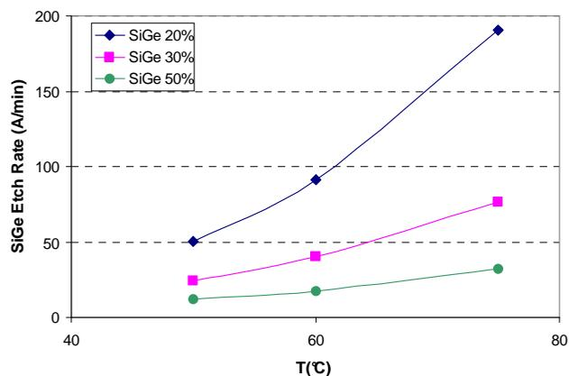
Fig.3. Evolution of the Si<sub>1-x</sub>Ge<sub>x</sub> (x: 0.2, 0.3 and 0.5) etch rates as a function of the temperature using a 25% TMAH spin-on dispensed chemistry.
