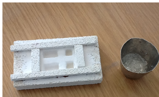
Figure 2. Molten glass-ceramic (transparent appearance) in platinum crucible and mold for the sealant test samples
